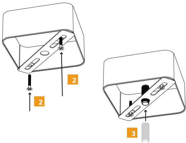
**6** Install the backplate of the fixture to the nipple with 1/8IP lock washer and 1/8IP nut.
